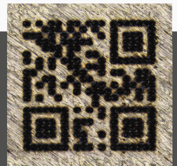
1mm by 1mm sized QR code marking on a brushed stainless steel sheet. (Bay Zoltán Nonprofit Ltd. for Applied Research)
