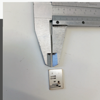
1mm by 1mm sized QR code marking on a brushed stainless steel sheet. (Bay Zoltán Nonprofit Ltd. for Applied Research)
