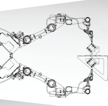
Lasram integrates industrial laser systems into robotic environment. With our metal 3D printing solution we provide high-precision robot automated manufacturing process for fast and efficient component production. Lasram's multi-robot configuration, utilizing the unique and patented Multidimensional Additive Production (MAP) technology of DUPLEX 3D in combination with WAAM, unlocks new opportunities in metal manufacturing.
