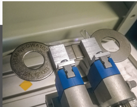
Automated laser marking and laser welding process of sheet metal parts.
