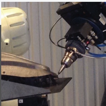
3D laser cutting of complex pressed sheet metal automotive part.
