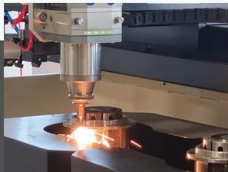
Automated 2D laser cutting of hardened steel clutch workpiece for ZF automotive industry supplier.
